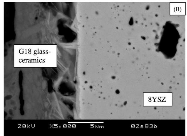
Fig. 5. Interfacial microstructure of the hybrid mica seal with G18 glass-ceramic inter-layers pressed between a metal pipe and an 8YSZ substrate at 800  $^{\circ}\text{C}$ , with an applied load of 100 psi for 650 h in air: (A) a low magnification, and (B) a high magnification at the interface.
