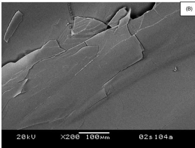
Fig. 4. Interfacial microstructure of the hybrid mica seal with silver inter-layers pressed between a metal pipe and an 8YSZ substrate at 800  $^{\circ}\text{C}$ , with an applied load of 100 psi for 324 h in air. The section under compression (A) clearly shows the diffusion of Ag into the mica and caused discoloration as compared to the section not under compression (B).
