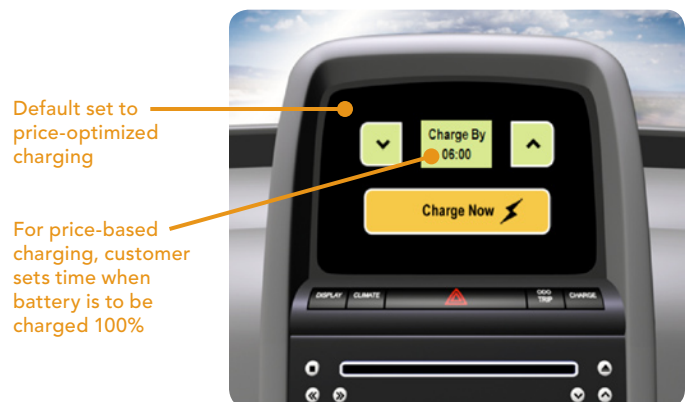
Smart Charger Vehicle Panel
