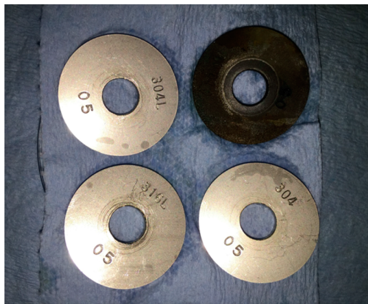
Figure 34. Steel coupons from ION's regenerator after 1100 h of testing. 157
