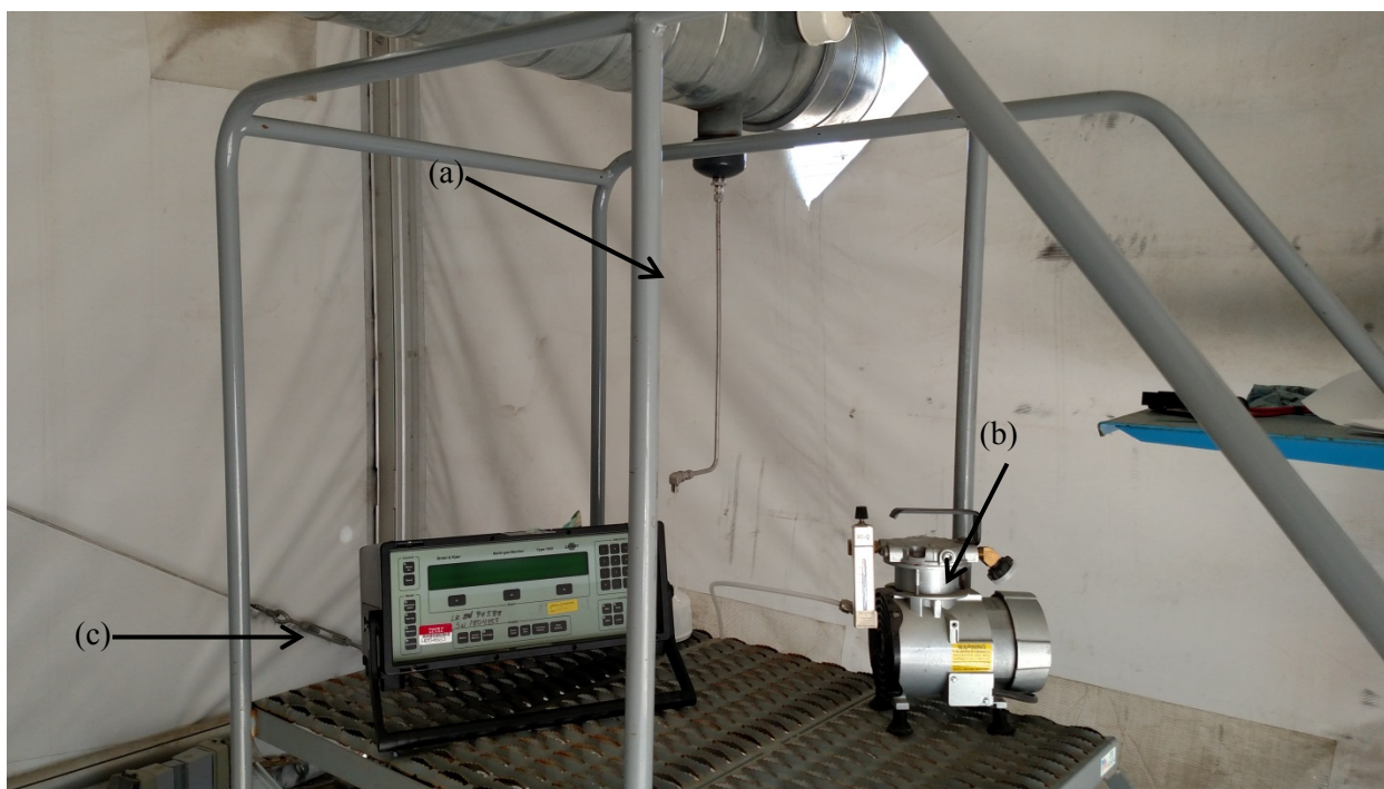
Figure 3.6. Equipment Used for the Gaseous Tracer Sampling: (a) Sampling Probe Installed in a Port, (b) Sampling Pump, and (c) Gas Analyzer
