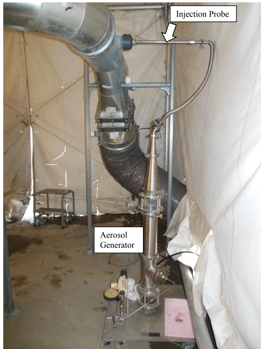
Figure 3.7. Equipment Used for Particle Injection
