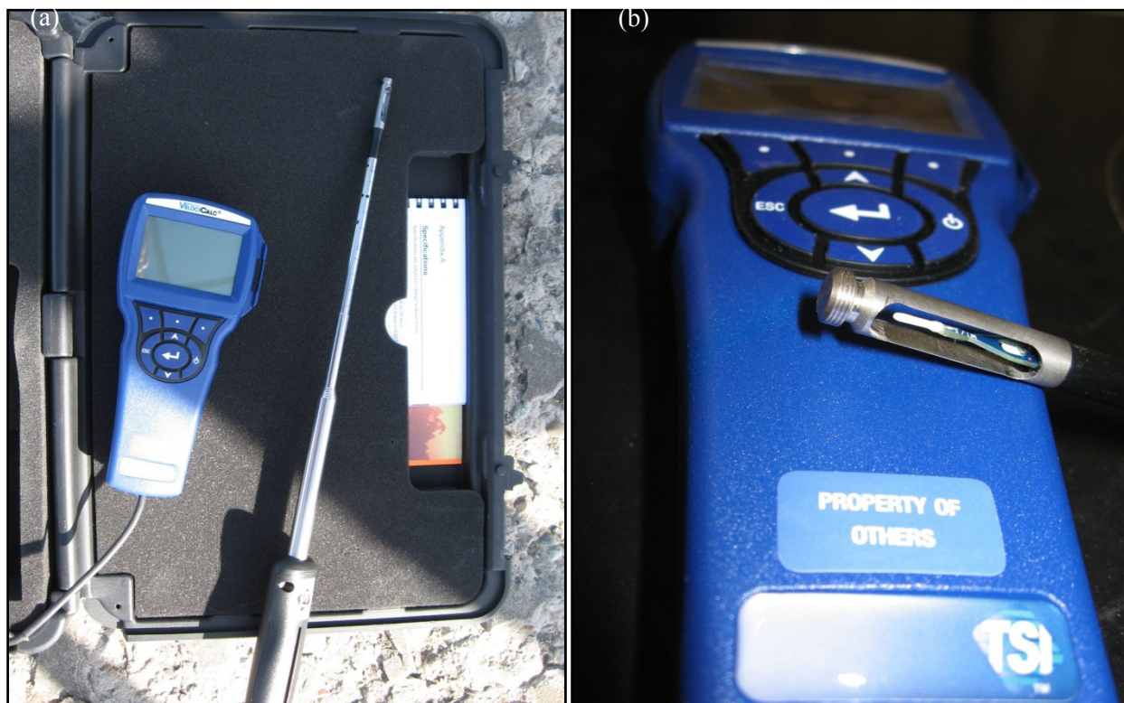
Figure 3.2. Equipment Used for the Velocity Uniformity Test (a) Thermal Anemometer, and (b) Close-Up View of Thermal Anemometer Probe Tip
