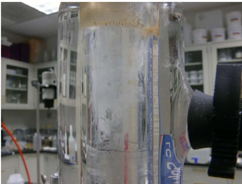
Figure 4.32. Debris Stuck to Column C after Testing at 75°C
