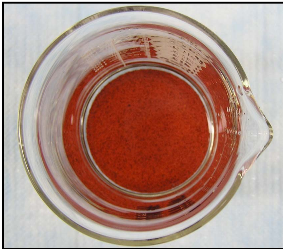
Figure 3.1. Representative SRF Resin Sample for Column Testing Showing Darkened Resin Beads
