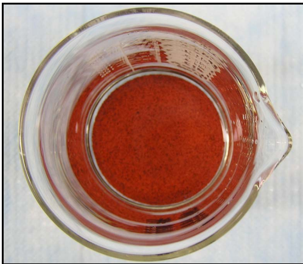
Figure 3.1. Representative SRF Resin Sample Showing Darkened Resin Beads
