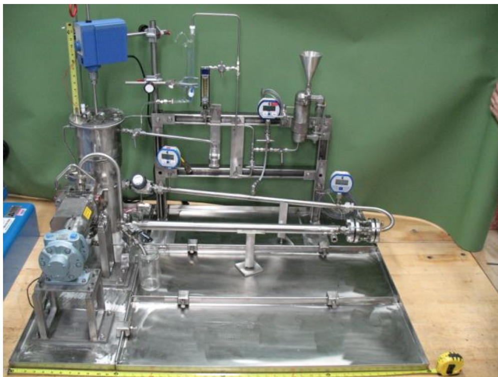
Figure 2.5. CUF Testing Apparatus before Hot Cell Installation
