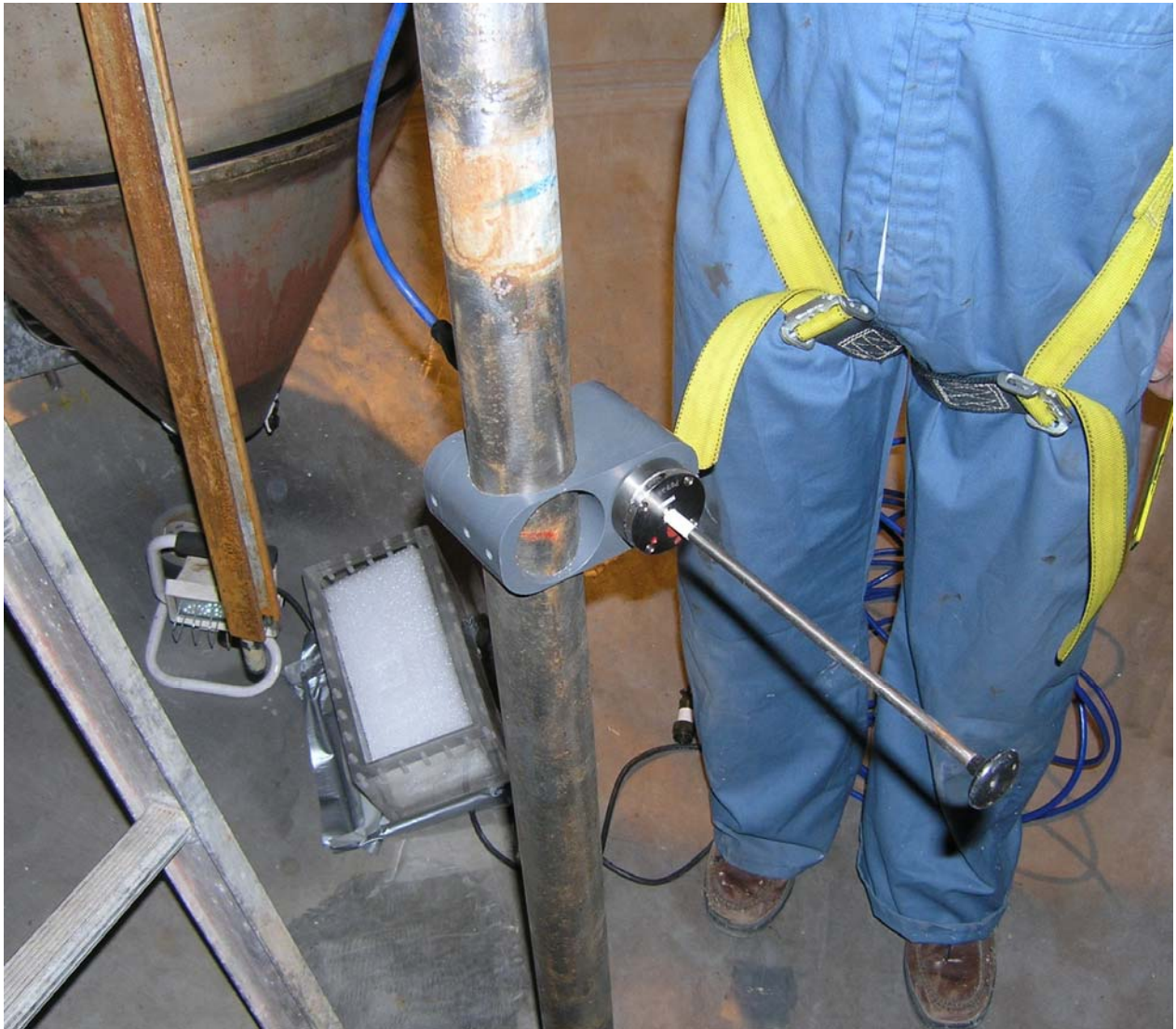
Figure 3.3. Velocity Probe Inside the Tank (in the 4-PJM configuration) at an Early Stage of the Installation. (It is not in the final position.)
