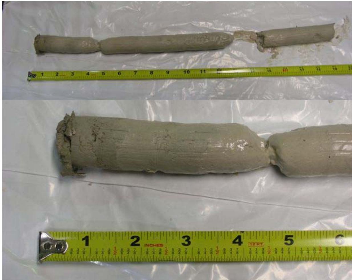
Figure B.2. Partial Section of a Clay Plug from a Sparge Tube
