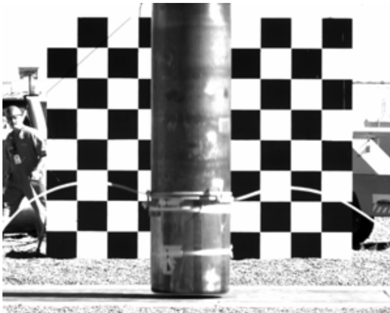
Canister HT503 viewed from southern camera immediately before impact.
