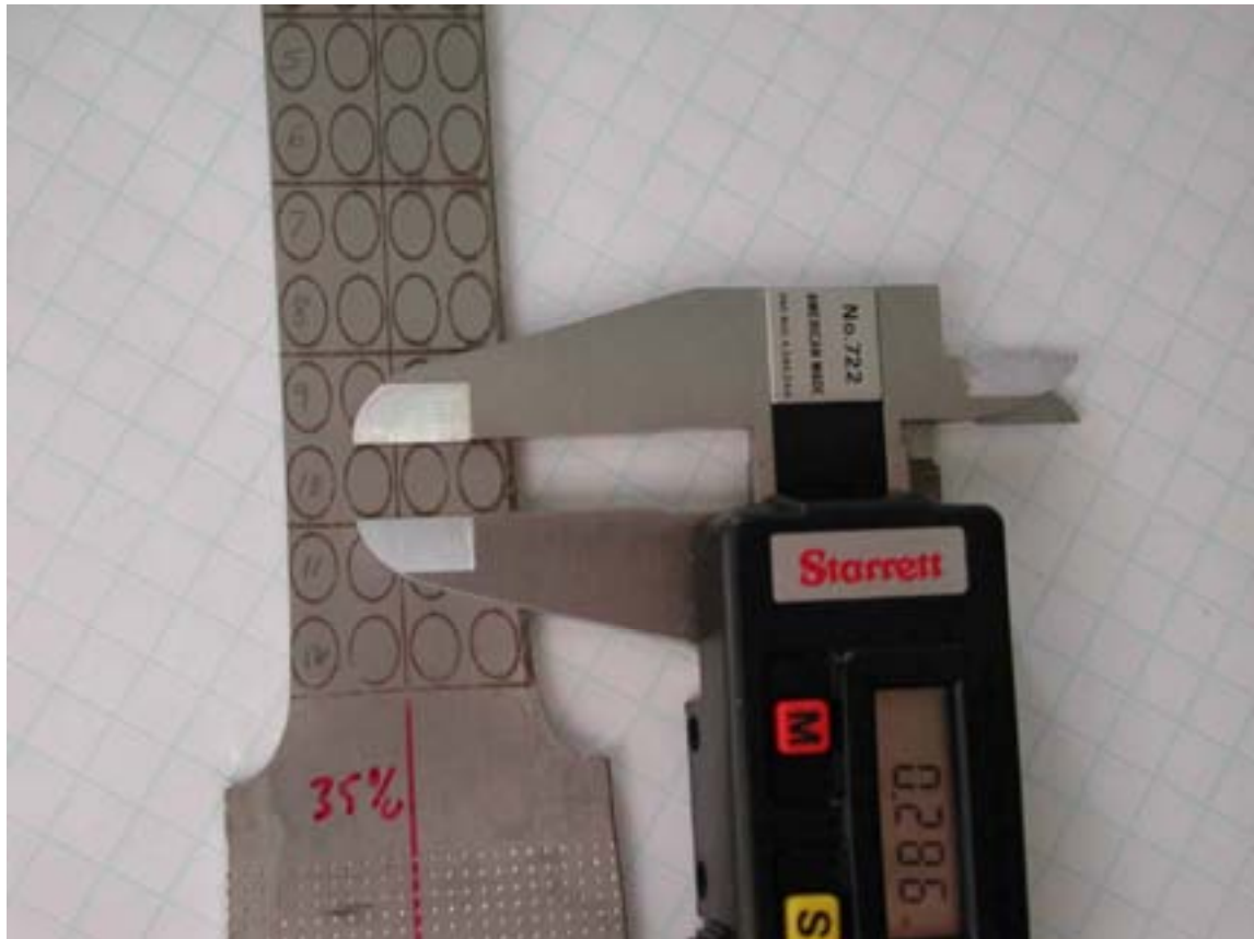
Figure I.4. Measuring Strain Circle with Caliper
