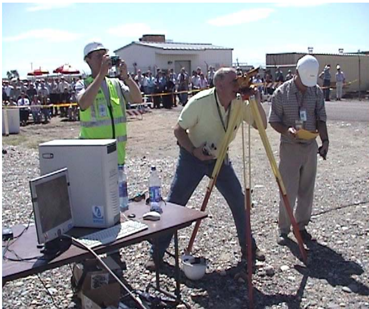
Figure 2.6. Canister Swing Verified to be Within 0.66 Degrees Using Two Transits Viewing the Canister from Perpendicular Angles
