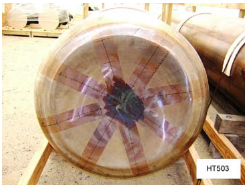
Bottom of HT503 (10-gage wall) after drop
