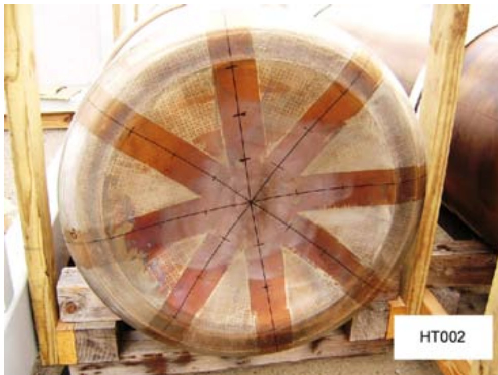
Bottom of HT002 (3/8-in. wall) after drop
