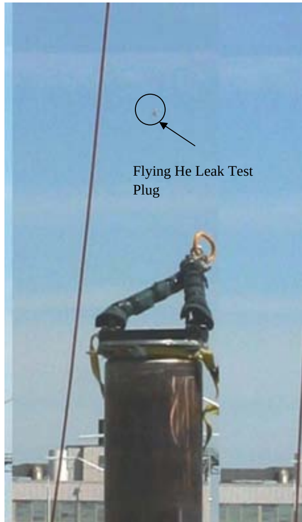
Figure 3.3. Helium Leak Test Plug Ejected Upon Impact During First Drop Test
