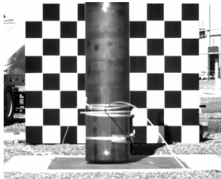
Canister HT503 viewed from eastern camera immediately before impact.
