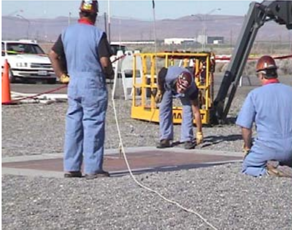
Figure 2.10. Canister Drop Height Established with Pre-Measured Tape and Plumb Bob
