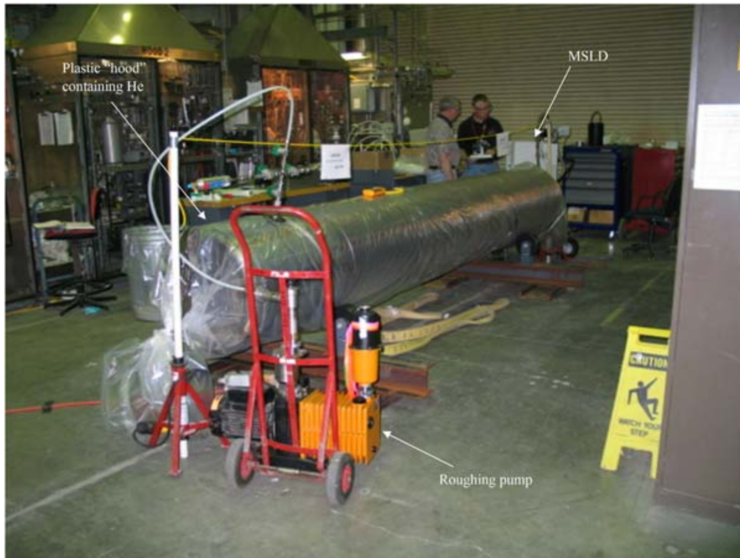
Figure 3.2. Helium Leak Check Using “Hood” Technique
