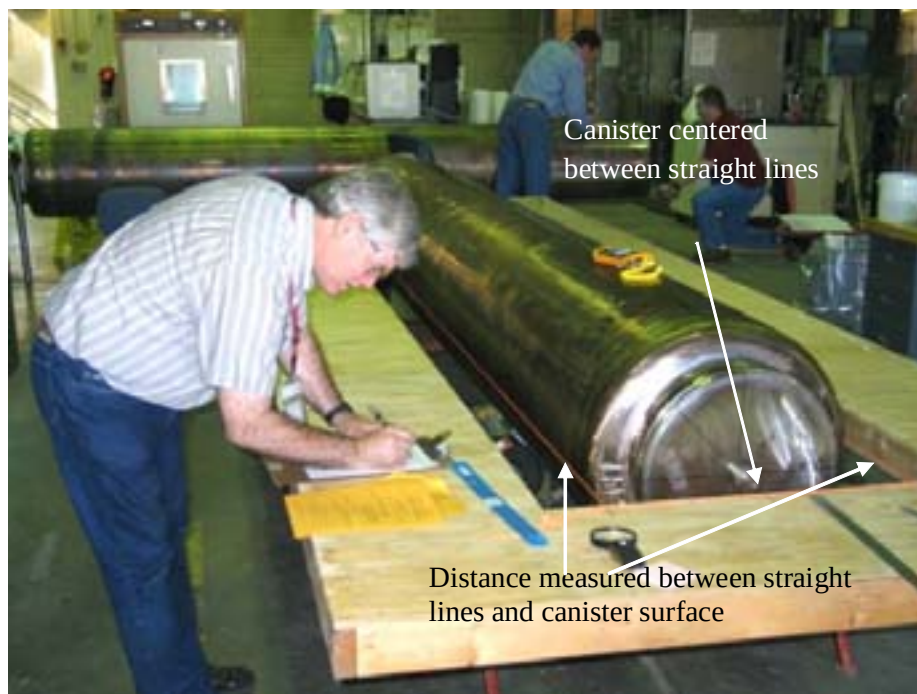
Figure 4.4. Measuring Bow and Warp Using Template with Straight Lines
