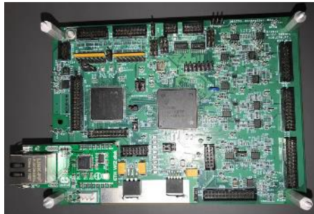
ORNL-Developed Commercialized DSP Controller Employing Ethernet Port
