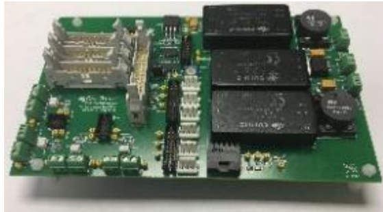
ORNL-Developed Universal Inverter Interface
