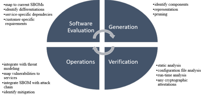
Fig. 1: The four phases of the SBOM lifecycle.
