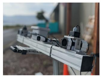
The easy-to-assemble technology uses a pair of thermal motion cameras to remotely sense movement of animals and objects in real time using a thermal signature.
