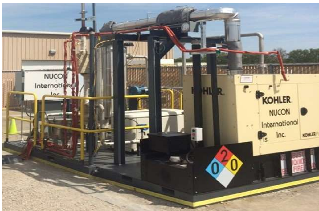
Fig. 1. Engineering-Scale Configuration of the TOS used in Phase 2 Testing at PNNL.
