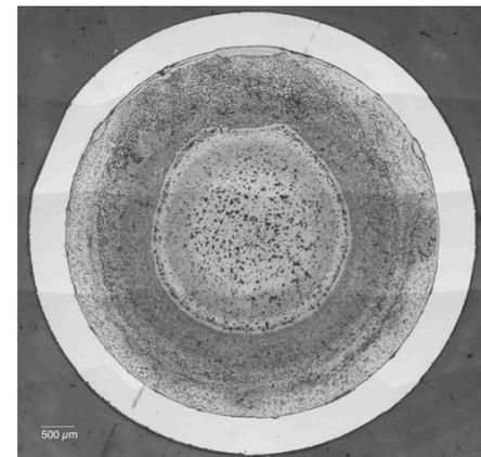
Metal Fuel with HT9 Clad
