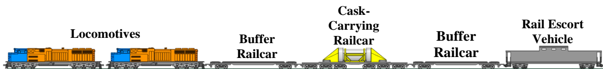
Fig. 1 Simplified Train Consist for Spent Nuclear Fuel Transport
