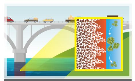
PNNL's SLIC Foul-Release Coating provides extended protection from harmful biofouling and can be used on critical infrastructure, maritime ships, ocean-rigging platforms, hydroelectric powerplants, as well as in food, agriculture, and medical environments.
