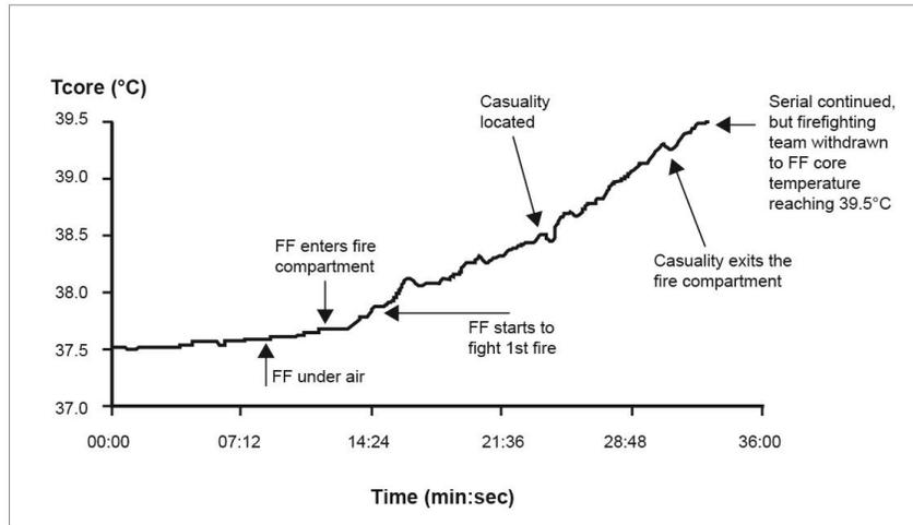
**Figure 5. Rise in core temperature during firefighting. (United Kingdom, 2005)**
