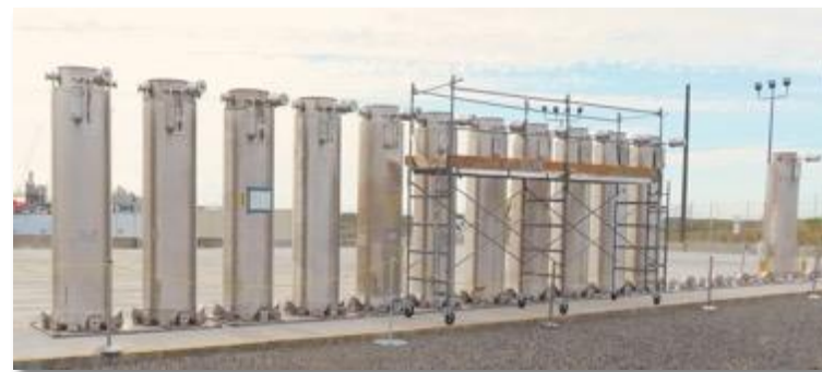
Twelve Loaded Ion Exchange Columns on Storage Pad, 587,000 curies of cesium-137
