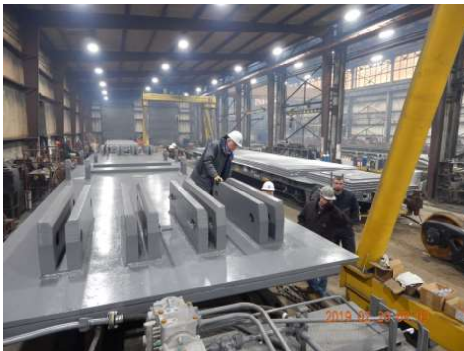
Fig. 6. Inspecting Atlas Railcar End Stop Pin Blocks (February 2019)
