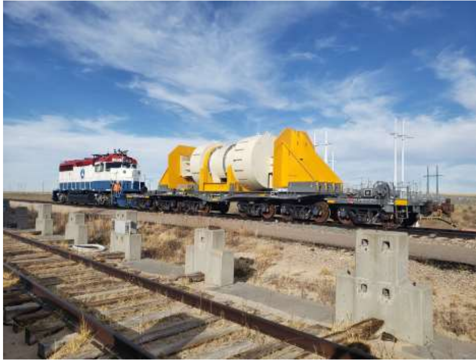
Fig. 7. Atlas Railcar with Heavy Test Load at TTC (October 2019)
