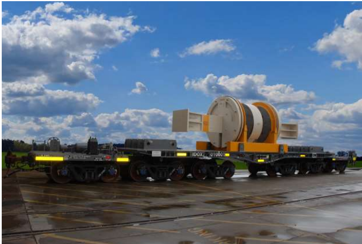
Fig. 8. Atlas Railcar with Minimum Test Load at TTC (October 2019)
