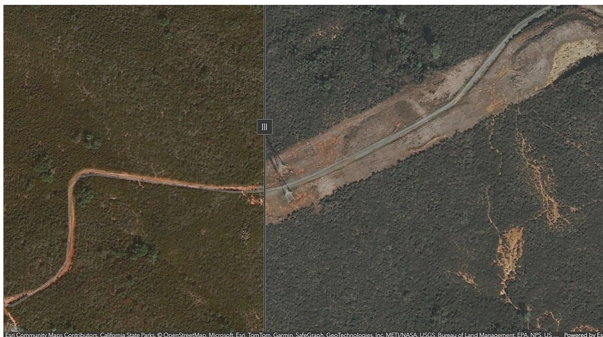
Figure 6. Before and after aerial view of the ROW where mastication took place. Left side shows the ROW before the land was cleared (June 2020). Right side shows the ROW after mastication took place (November 2021).
