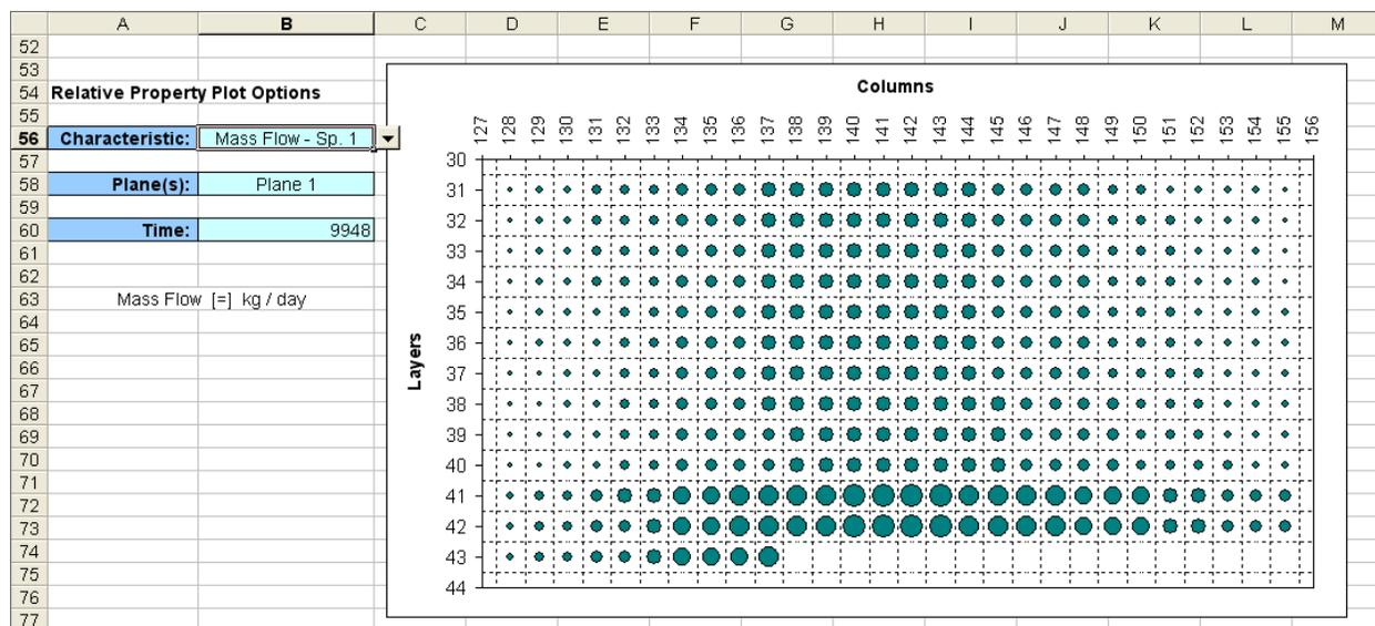
**Figure 4.** Example of a Bubble Plot Showing the Relative Magnitude of Mass Flow Rate for a Specified Plane at a Particular Time Point in the Simulation — Drop down lists allow the user to select the property (also including volumetric flowrate and concentration), plane, and time to display. The bubble sizes are scaled relative to the largest value in the simulation so that the size shows the proper relative magnitude when looking at different time points.
