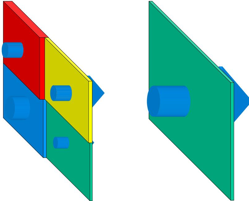
**Figure 9.** *Depiction of Mass Flow Through the Grid Cells That Comprise an Entire Plane — The total mass to pass across the plane of a grid cell (depicted by the thickness of the boxes) may vary because of differences in volumetric flow rate (size of arrows) resulting from aquifer heterogeneity and/or hydraulic stresses and differences in concentration (color of boxes with red = high, blue = low).*
