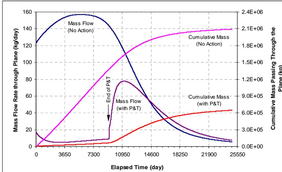
**Figure 26.** Mass Flow Rate and Cumulative Mass to Pass Through a Plane for the Two Scenarios of the Multilayer Example — In one case no action is taken (natural attenuation only) and in the other P&T is applied. In both cases, the non-aqueous phase liquid source was removed.
