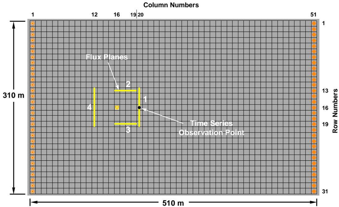
**Figure 11.** Locations of the Four Flux Planes Used in the Simple Example and the Observation Point for Time Series Concentration Plots
