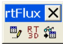
**Figure 1.** *Toolbar for the rtFlux Utility — From left to right the toolbar buttons are: Modify the BTN File to Incorporate Flux Plane Definition(s), Run RT3D, and Process Flux Output and Read Into Excel.*
