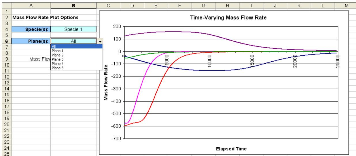
**Figure 3.** The Time-Varying Mass Flow Rate Plot on the "Graphs" Worksheet — The user may select which species and which plane to view (including all at once) via drop-down selection lists. The cumulative mass flowing through the plane plot is also on the "Graphs" worksheet and is configured similarly.
