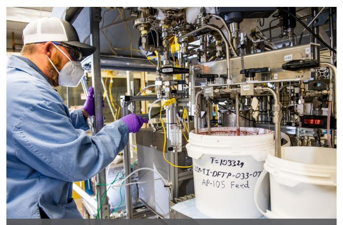
One of the many ways PNNL researchers support Hanford Site operations is by running simulated tank waste in a Continuous Laboratory Scale Melter in the Wasteform Development Laboratory—prior to running actual Hanford tank waste through similar equipment in the Radiochemical Processing Laboratory. Pictured on the cover is the viewport where researchers observe the cold cap, which is the slurry that floats on the molten glass before it has fully reacted. *Photo by Andrea Starr | PNNL*
