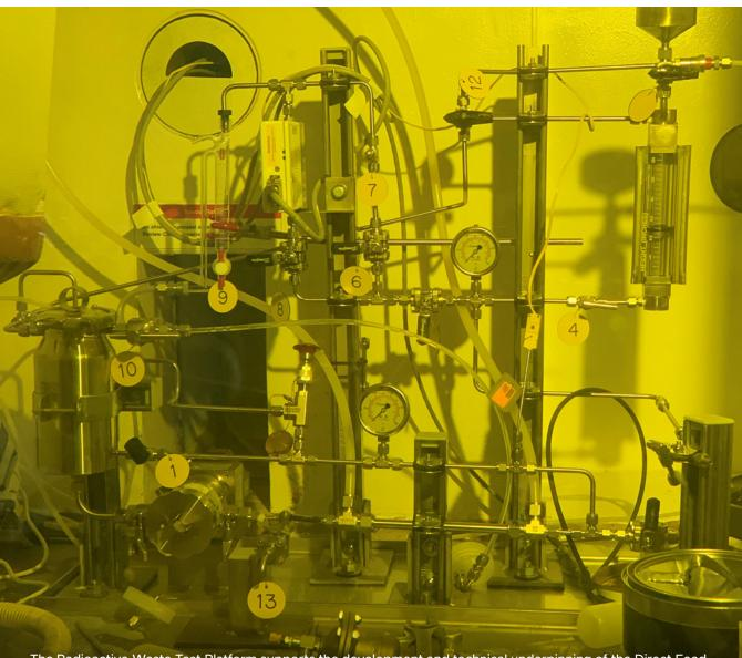
The Radioactive Waste Test Platform supports the development and technical underpinning of the Direct Feed Low-Activity Waste baseline flowsheet—including filtration, ion exchange, melter, and evaporator operations—reducing risk and efficiently providing solutions to any emerging tank waste processing operational issues.
