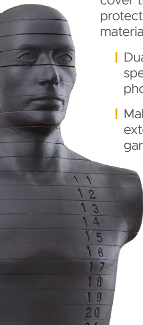
Anthropomorphic phantoms with internal cavities for thermoluminescent dosimeters (TLDs)
