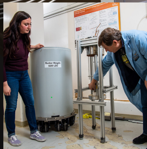
Lead Shielded Gamma Bunker
