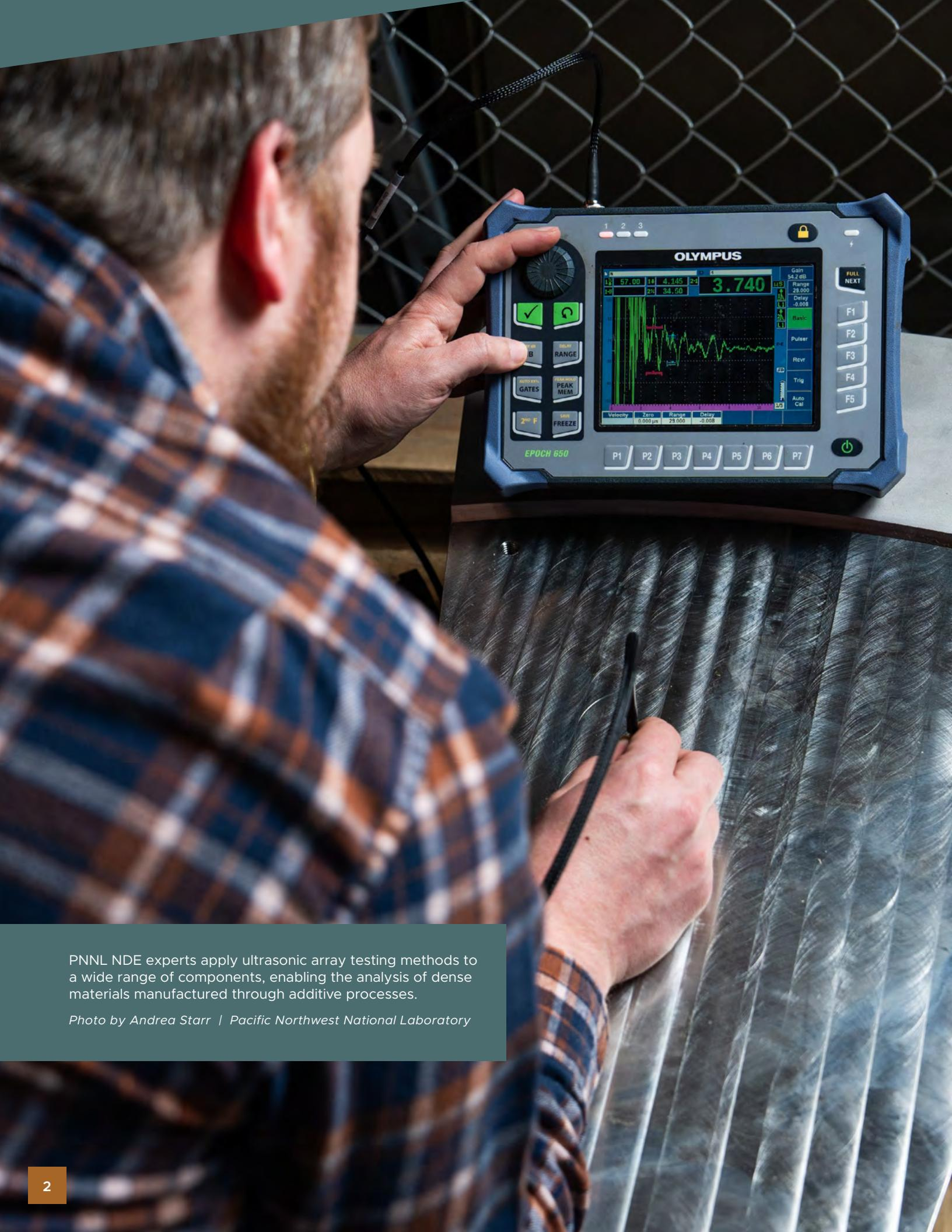
PNNL NDE experts apply ultrasonic array testing methods to a wide range of components, enabling the analysis of dense materials manufactured through additive processes.
