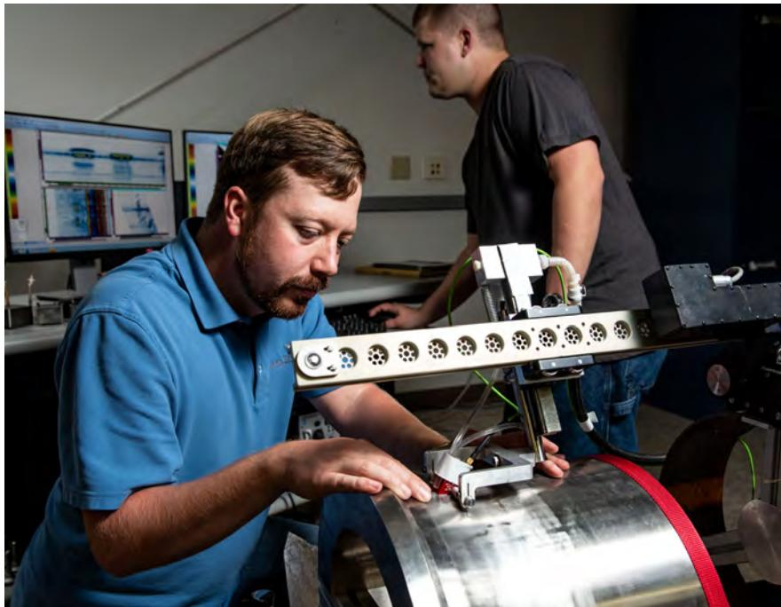
NDE experts at PNNL apply ultrasonic testing methods to a wide range of components, enabling the analysis of dense materials manufactured through additive processes.
