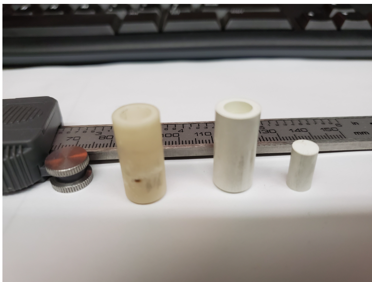
Figure 2.2. \text{Al}_2\text{O}_3 and BN crucibles for testing thermal expansion and calculating density with a TMA.
