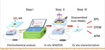
*E*-Cell is a three-step process that includes electrochemical analysis, in-situ SEM/EDS, and EX-situ characterization.
