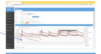
By selecting a time interval on the data chart, — integral emission values are computed
