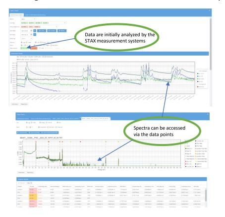
Emission values are calculated independently by the STAX measurement system and on the STAX server. Significant deviations between the results are indicated by vertical bars for quality control
