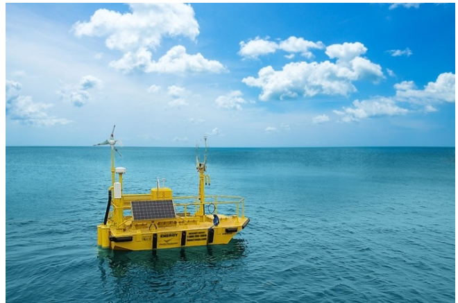
Department of Energy lidar buoy deployed off the coast of California (Photo by: AXYS Technologies, Inc.)
