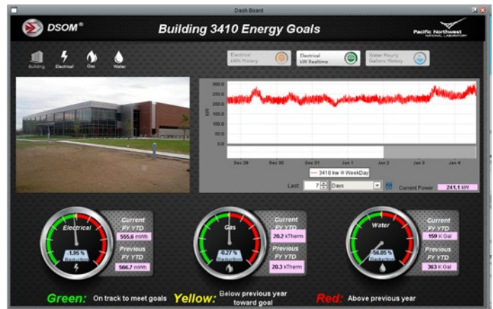
DSOM dashboard showing electrical, gas, and water consumption at a Pacific Northwest National Laboratory building.
