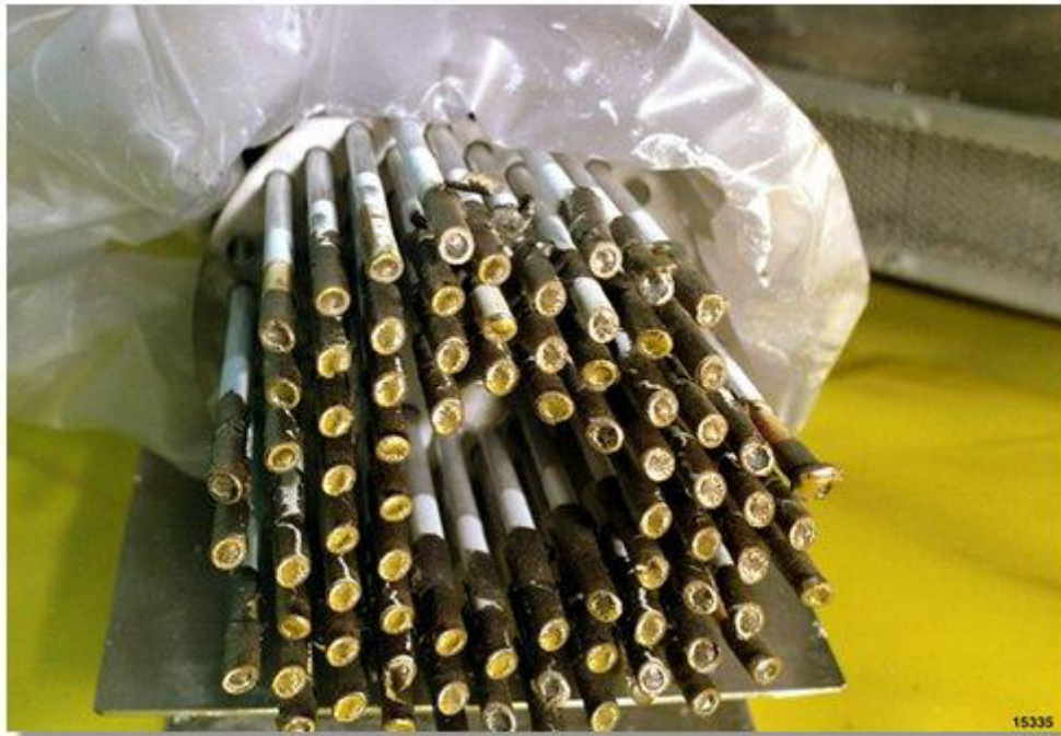
Figure C.27 Metal fuel after casting
