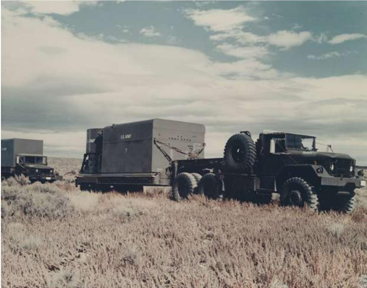
Fig 2. Full-Scale Mockup of the ML-1 Nuclear Power Plant
