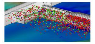
This software tool accurately and efficiently estimates the time sequence of 3D locations of fish tagged with transmitters. It collects enough detail to assess the function of dam-passage design alternatives, for example. It estimates a fish's location by calculating the time difference of arrival from all hydrophones that detect the transmission from the tag on that fish. During field tests at several dams, 3D Tracking V2.0 performed significantly better than other available solvers.
