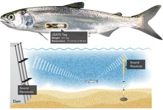
PNNL's acoustic telemetry tags release beeps, unique to each tagged fish. Receivers placed in rivers, lakes, or other waterbodies receive the signals as the tagged fish swim by, and collect data that help researchers map the precise 3D location of each fish and determine if those fish were injured during their travels.
