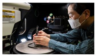
Materials scientist Dr. Guosheng Li uses the Zeiss X-ray microscope system (Versa 610) to obtain high-resolution, three-dimensional images of materials and devices of various size and format through a non-destructive, non-contact mode.
