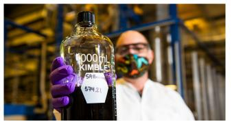
Chemical engineer Alan Zacher holds a jar of human waste after going through thermal liquefaction. The waste-to-biofuel project is in partnership with Greater Lakes Water Authority and sponsored by the U.S. Department of Energy's Bioenergy Technology Office.
