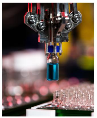
High-Throughput Experimentation System robotic systems are used for high-throughput experimentation for material synthesis preparation. The systems realize high-throughput studies of large material groups by using design experiment concepts combined with machine learning and small-scale testing.
