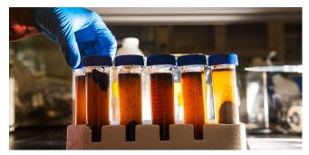
Tubes of fine soil particles are seen separating within the sodium polytungstate mixture; light particles are floating on top, while heavy particles are sinking to the bottom of the tub. Sodium polytungstate is a compound that remains in a liquid form even after it's very dense. The solution is 2.5 times the density of water and is commonly used to separate heavier particles from lighter ones.
