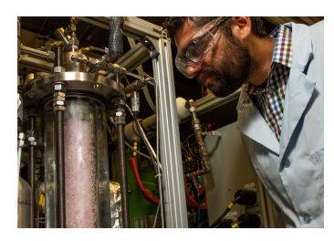
PNNL researchers use custom-built systems like this one to parametrize and validate models of how solvents and  ${\rm CO_2}$  move through packing materials.
