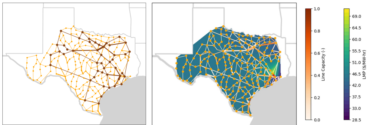
Figure 7. The 200-bus transmission network (left), with 345 kV lines shown in brown and 138 kV lines in orange. The line thickness is proportional to its MVA rating. Resulting line congestion (denoted by the line color) and geographic variation in LMPs are shown on right.
