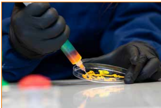
ArtSea Inks can be added throughout the printing process using a nozzle to apply different colors, or the material can be colored prior to printing.
