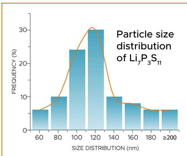
*With PNNL's synthesis method, particle sizes for sulfide solid electrolytes can be easily manipulated down to tens of nanometers.*
