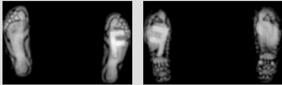
Example mm-wave image of person-worn footwear.
