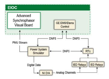
PRIME translates simulated data into analog signals that real-world hardware can understand and respond to. Hardware responses are linked back to create a closed-loop simulation that alters the underlying power system simulation. This allows for real-time, interactive visualization of advanced applications, realistic cyber red team exercises, and remote hardware testing using industry standard interfaces.
