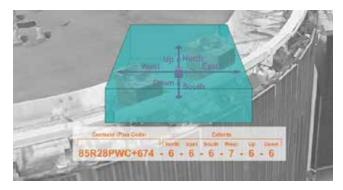
A unique code string identifies a space and its extent, enabling Identify n-D to cross-reference various spatial data in less than a millisecond with nearly double the accuracy.
