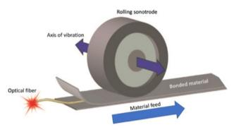
This illustration depicts a rolling ultrasonic welder bonding, an optical fiber sensor between two metal foils. PNNL's monitoring technology makes it more reliable to manufacture bonds around embedded sensors. The sensors themselves can be used to confirm that the weld was completed successfully.
