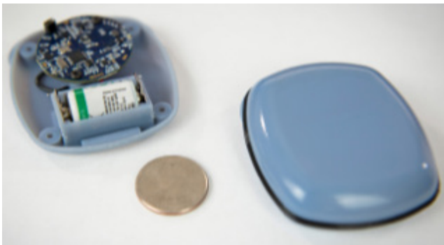
PNNL designed the R&D 100 Award-winning Acoustic Gunshot Detection technology to be easily adapted and affordable. The golf ball-sized sensor contains a Wi-Fi-enabled microcontroller, microphone, and battery.
