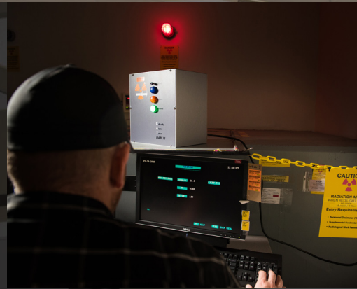
Criticality Safety Alarm being tested with a neutron irradiation well
