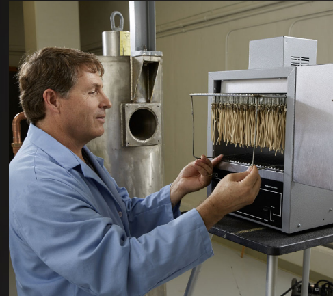
Combined radiation and temperature effects testing of electrical insulation
