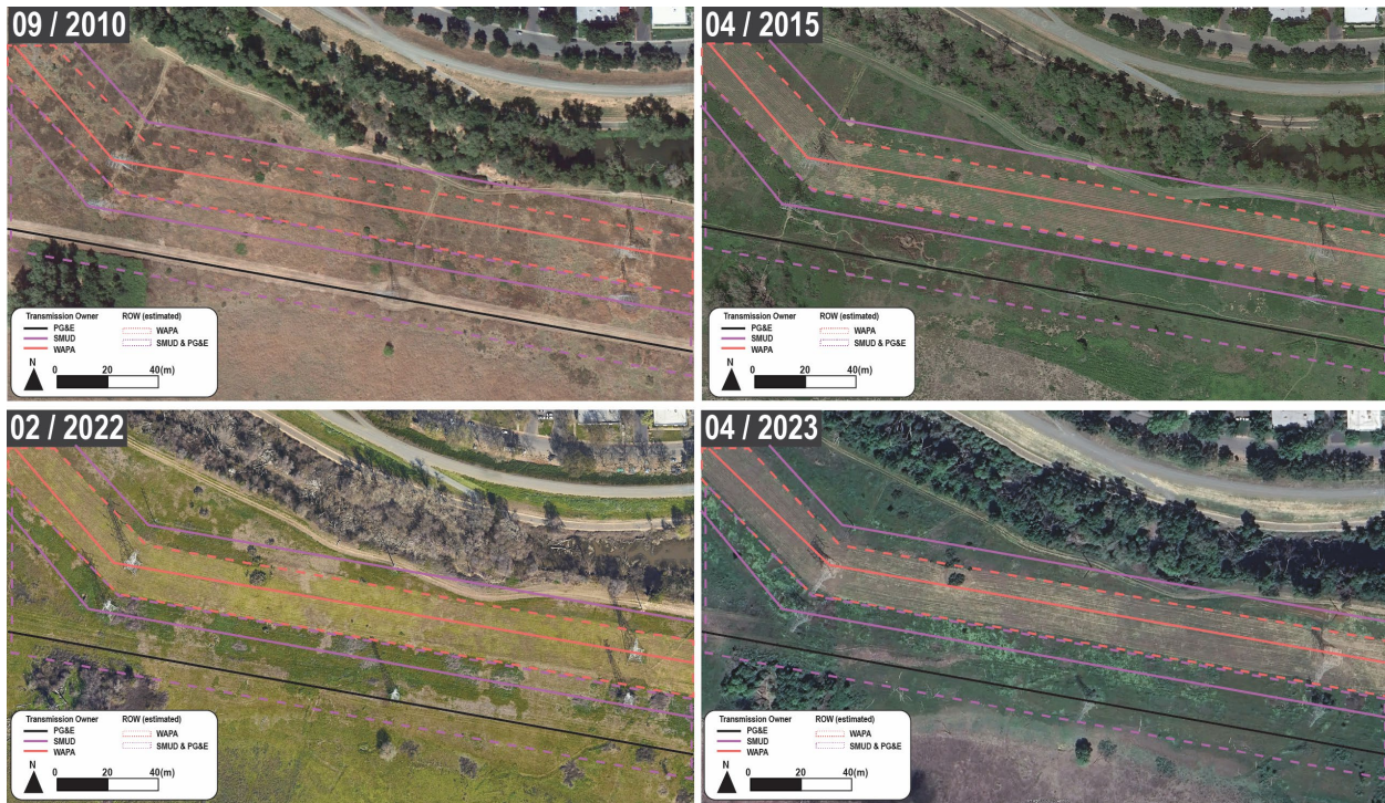
Figure 5. SMUD and PG&E share a transmission corridor in the Parkway, and WAPA, a federal entity, has a parallel transmission corridor. Utilities implement different management practices in their ROWs as demonstrated here, where mowing is used to remove vegetation in WAPA's corridors, whereas IVM is implemented in SMUD and PG&E's corridors, as evidenced by the low-growing vegetation.
