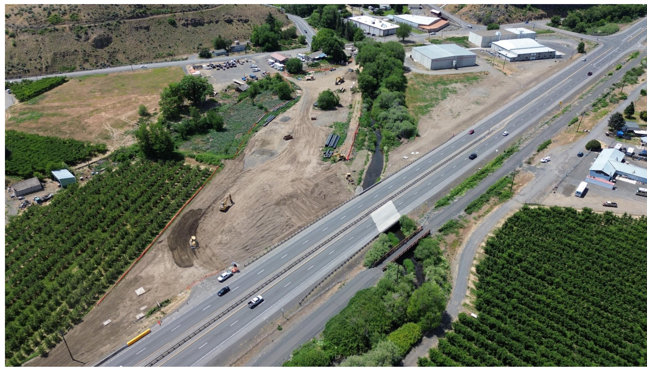
Fig 5. Yakima County's Cowiche Creek levee setback project, in conjunction with the City of Yakima's Nelson Pipeline project will install a pump station on the landward side of the levee powered from the power pole (bottom left), and power to the Naches Cowiche Canal Company shop will be rerouted to higher ground. (Kory Graafstra, Yakima County).
