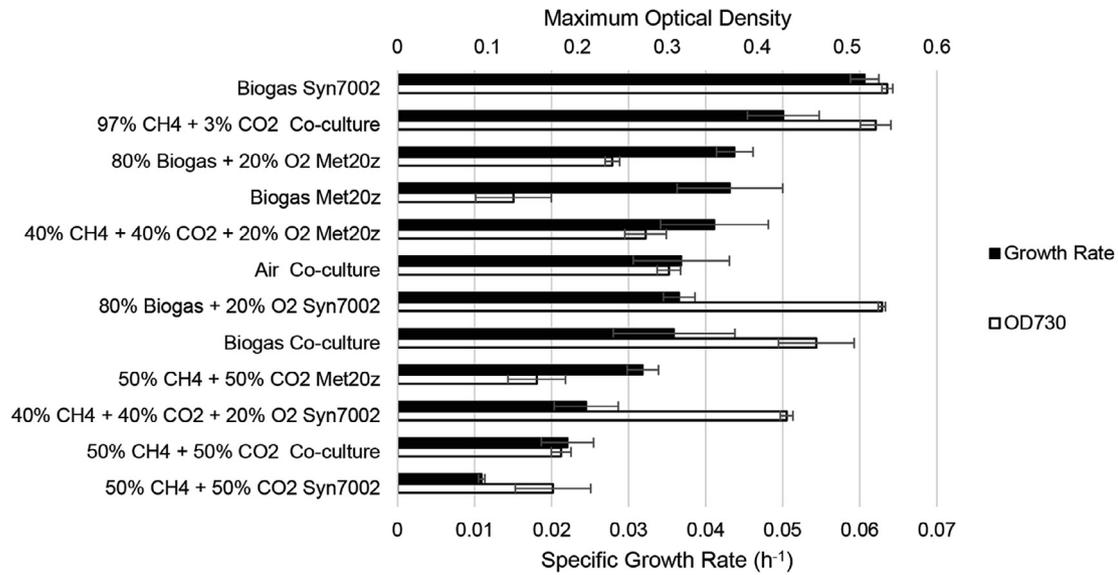
**Fig. 2.** Batch growth performance on variable gas mixtures used as the sole carbon source for the co-culture and axenic controls of *M. alcaliphilum* (Met20z) and *Synechococcus* 7002 (Syn7002), respectively. Each data point represents the mean of triplicate experimental measurements for either the specific growth rate or maximum optical density; error bars represent  $\pm 1$  standard deviation.
