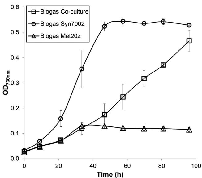
Fig. 1. Dynamics of batch growth supported on raw biogas used as the sole carbon source. Co-culture performance on biogas compared to axenic controls of *M. alcaliphilum* (Met20z) and *Synechococcus* 7002 (Syn7002), respectively. Each data point represents the mean from triplicate experimental measurements of optical density; error bars represent  $\pm 1$  standard deviation.
