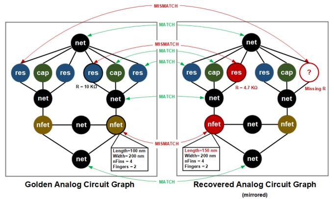
Fig. 4. Example golden vs. recovered parametric graph isomorphism, showing a mismatch on one of the resistors, a match on two of the nets, and a mismatch on a parameter in one of the NFET devices. Mismatches can also be found in capacitance values, voltage nodes, etc.
