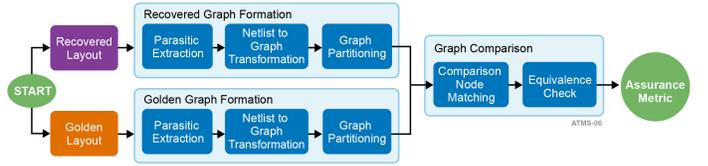
Fig. 3. Overview flow diagram showing the general flow of the analysis. Two layouts, one for the golden design and one for the recovered design, are ingested into a PEX tool to produce a SPICE netlist. That SPICE netlist is transformed into GraphML and undergoes graph partitioning to reduce the complexity of the search space. The resulting graphs are then digested by PGI to perform the final comparison and equivalence checks to find deviations in the recovered.
