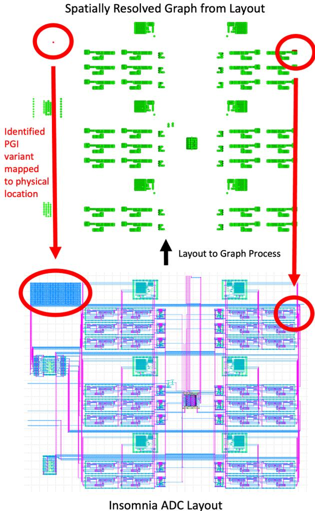
Fig. 7. ADC Variant layout (shown at the bottom) contrasted with the PGI generated graph (shown at the top) showed the approximate location of the variant that have been marked due to parameters being out of tolerance. The left most circle is the actual wire that the variant changed. The right most circle is the effect the variant had on the connectivity of the layout.
