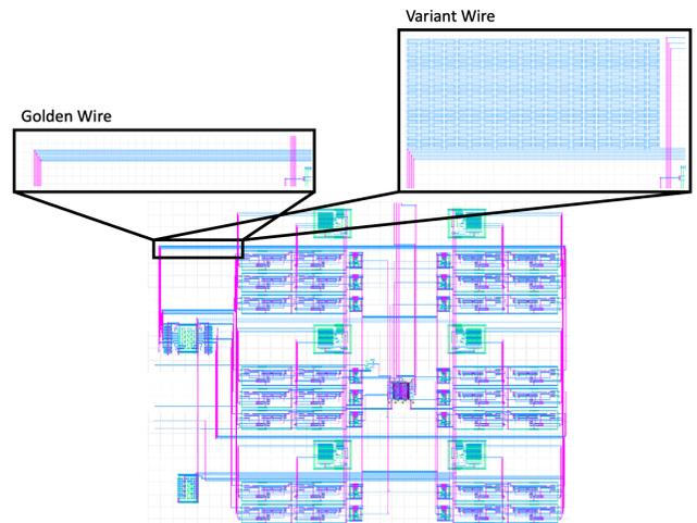
Fig. 6. ADC Variant layout showing both the golden and variant versions of the affected wire.
