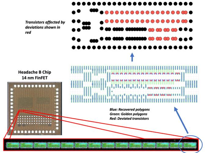
Fig. 5. Headache B was ingested into the CHARGE framework and analyzed against Headache A for deviations in the AMS/RF circuitry. One stage of the ring oscillator is shown with the affected transistors in red and non-affected transistors in black due to the introduced deviations.
