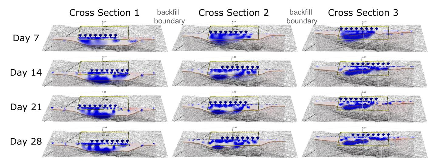
The presence of backfill material has a significant impact on the distribution of flush water to the Hanford Fm., and therefore on remediation performance.
