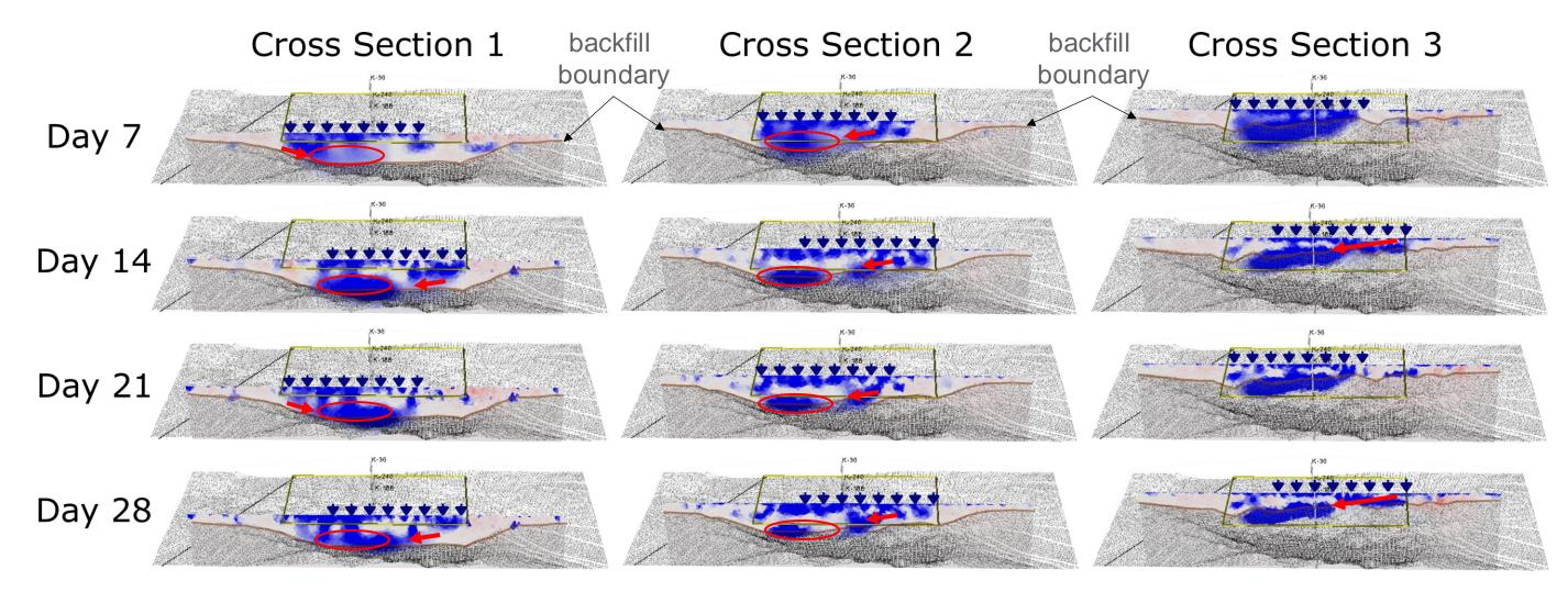
Flush water flows along backfill boundary with Hanford Fm., perches at deepest points, redistributes before flowing downward
