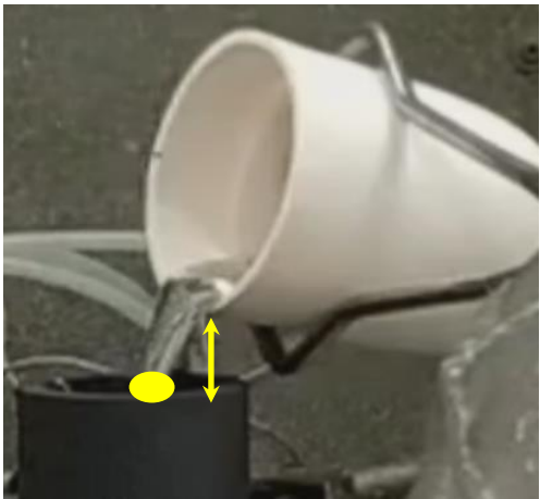
Mold-filling data (i.e., pouring area and flow rate) were obtained from experiments conducted at PNNL
